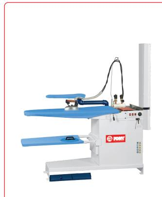
**GENUS-S** which features vacuum and hot air blowing from the large buck and can be supplied either with regular height fixed board or an adjustable height board from 770 mm to 970 mm utilising a gas spring.
